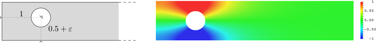
Figure 2.41: Left: geometry of the half waveguide. Right: real part of a trapped mode for \varepsilon = 0 and k^0 := \sqrt{\lambda^0} \approx 2.7403 . The computation has been realized by using Perfectly Matched Layers.
